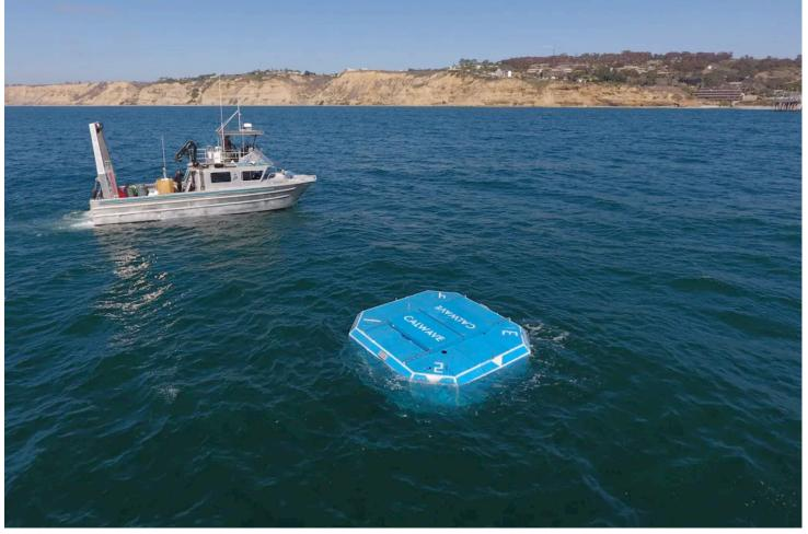
This type of wave-energy device is moored in the open ocean, where it is submerged. Units like this from CalWave will be used in a project off the coast of Oregon that will provide power to the grid. Photo courtesy of CalWave
